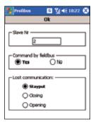
If a Profibus interface is detected on INTELLI+ by INTELLIPOCKET, the configuration window is available with the "Check/Bus" menu or "Change/Bus" menu. The following window is displayed.
