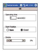
The partial stroke function permits to operate the actuator to a limited stroke. To use this function, several parameters are available:
