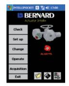
The main menu opening starts a connection attempt with an actuator. To communicate with INTELLI+, set up the actuator in local mode, and they got inferred connection of Parliat C. and activator force to force
